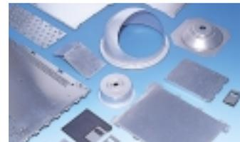
These functional resin coated aluminum sheets provide enhanced formability, corrosion resistance, scuff- and fingerprint-resistance, resistance to chemicals, electrical conductivity, ease of printing, and anti-bacterial and anti-mold properties. They are also self-lubricating, so that disposal of the lubricants and cleansers formerly used in the stamping process is eliminated.
