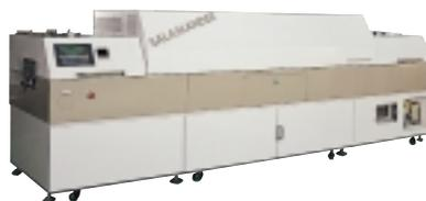
This reflow oven carries out the reflow soldering process during the mounting of electronic components in a nitrogen atmosphere. This eliminates the need to cleanse completed circuit boards, obviating the use of CFCs.
