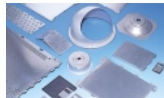
These functional resin coated aluminum sheets provide enhanced formability, corrosion resistance, scuff- and fingerprint-resistance, resistance to chemicals, electrical conductivity, ease of printing, and anti-bacterial and anti-mold properties. They are also self-lubricating, so that disposal of the lubricants and cleansers formerly used in the stamping process is eliminated.
