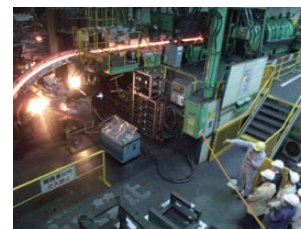
Mie Works : A close-up look at just-produced 1100°C copper rod
