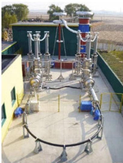
30m 275kV superconducting cable verification test (Shenyang)
