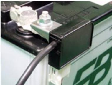
Lead battery status detection sensor installed in a vehicle
