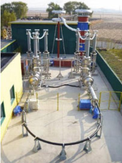
30m 275kV superconducting cable verification test (Shenyang)
