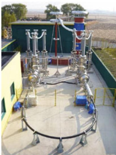
30m 275kV superconducting cable verification test (Shenyang)
