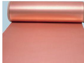
Electrodeposited copper foil
