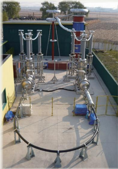
High-temperature super-conducting power cables
