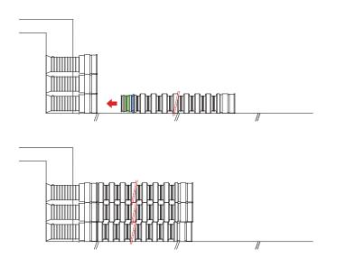
When the length in between the pipes from both ends of the handholes is shorter than the fixed pipe length, adjust to the required length, by using AQUA-Square.
