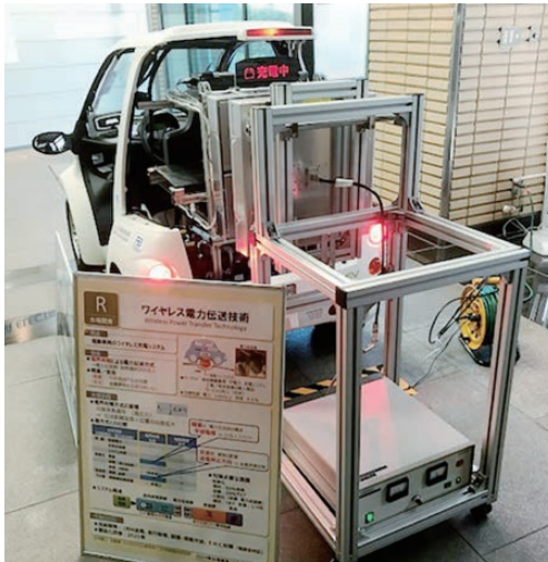
Figure 16 The electric field resonance coupler with a shield box mounted in a mobility car.
