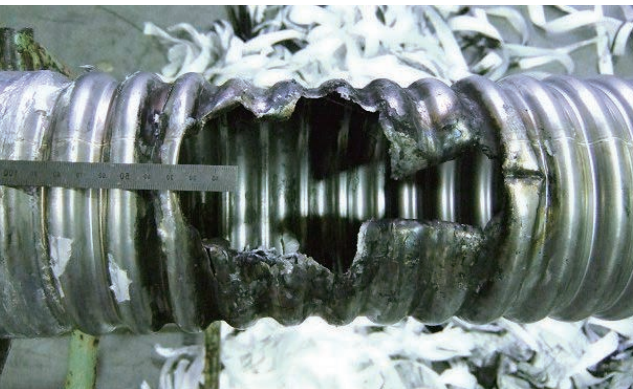
Figure 8 The Appearance of the damaged inner corrugated pipe.
