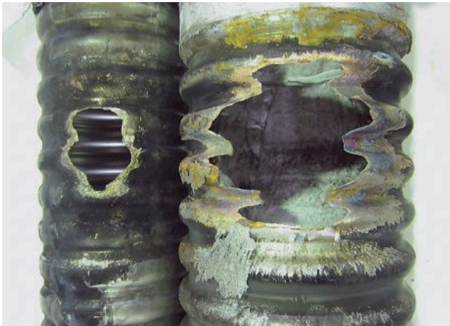
Figure 4 The Damaged appearance of the cryostat pipe with AC 10 kA. The left is the inner pipe and the right is the outer pipe.
