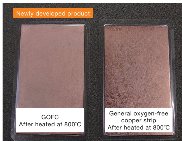
Figure 5 Appearance of the crystal structures kept at 800°C for one hour (in an argon gas atmosphere).
