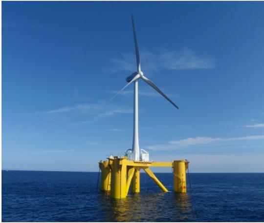
2MW Downwind-type Floating Wind Turbine
