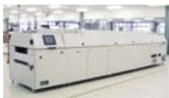
Reflow oven for use with lead-free solder
