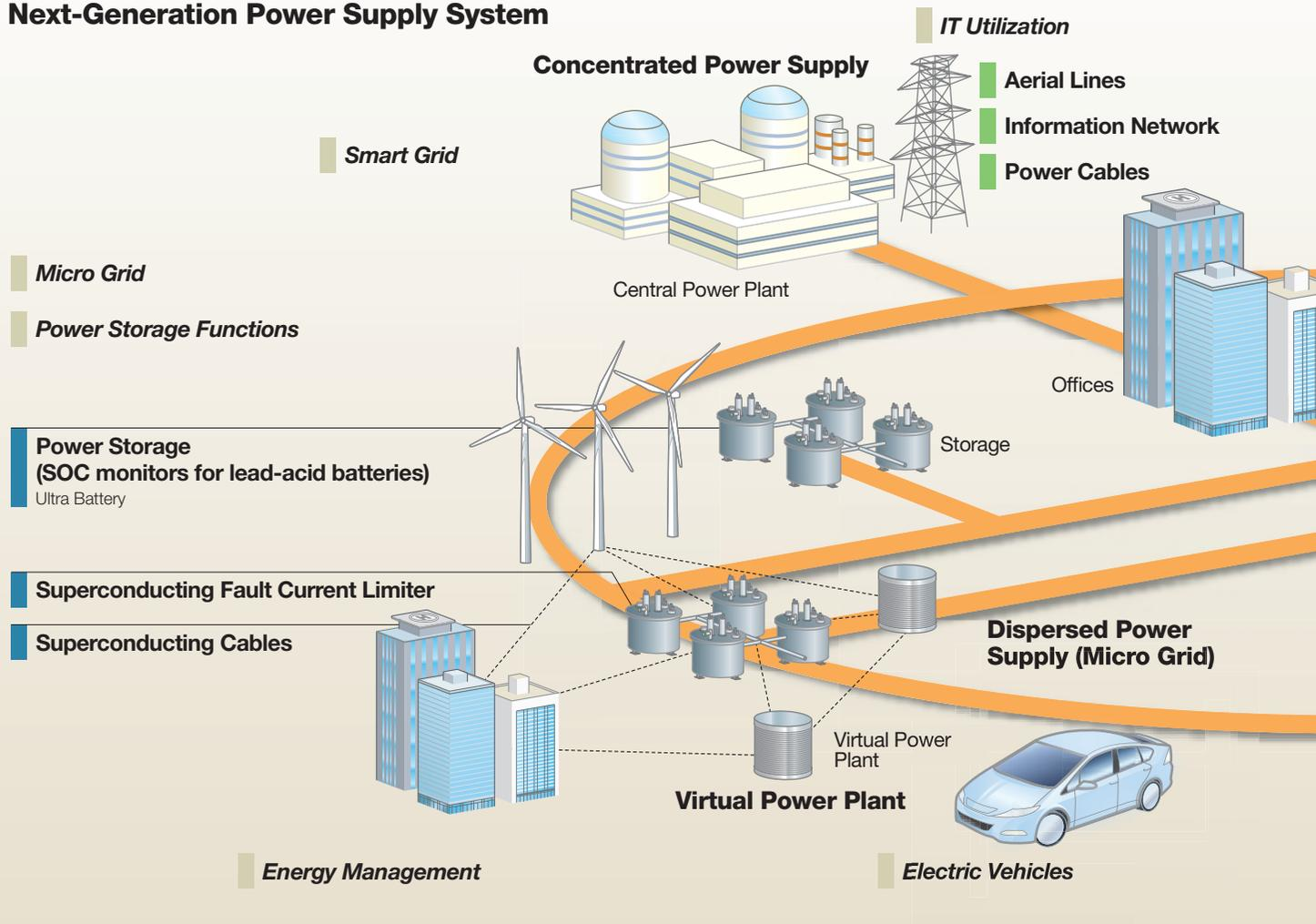
coordination with conventional energy sources. To coordinate these energy sources with new ones, Furukawa Electric is engaged in R&D of innovative control systems, comprised of power storage devices, power conditioners, and so on.
