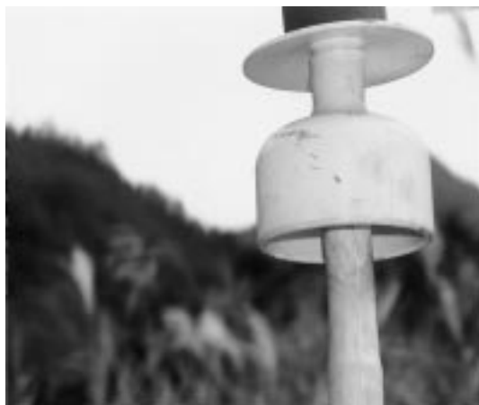
写真7 撤去品（中汚損地区:1年後） Sample after one-year outdoor exposure test in medium pollution area
