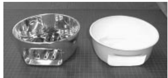
写真7 MCPET成形加工例(ダウンライト) MCPET vacuum thermoforming (Down-light)
