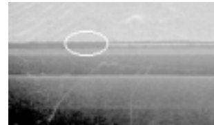
写真2 500 mW照射後のNDフィルタのSEM写真 SEM image of ND filter after 500 mW optical power incidence
