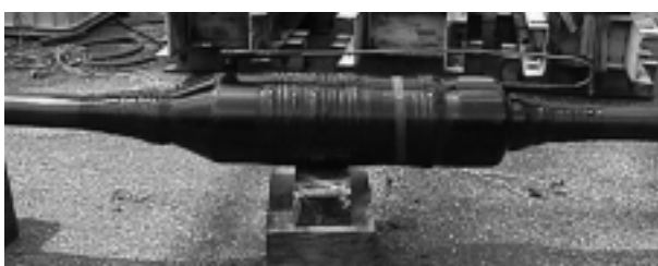
写真3 開発試験供試CSJ Specimen CSJ for long term test
