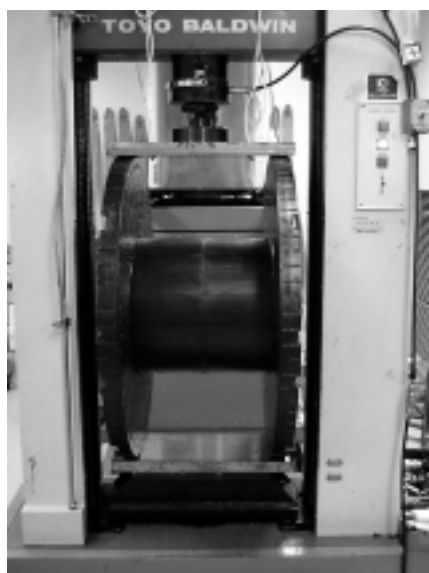
写真4 鏢圧縮試験 Determination of flange compression strength
