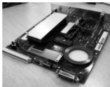
図17 PMD補償器の外観 Appearance of PMD compensator
