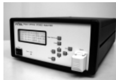
図5 高精度DOP測定器の外観図 Appearance of high precision DOP measuring instrument
