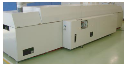
写真6 一体型窒素発生装置 Appearance of nitrogen separating system integrated with main oven.
