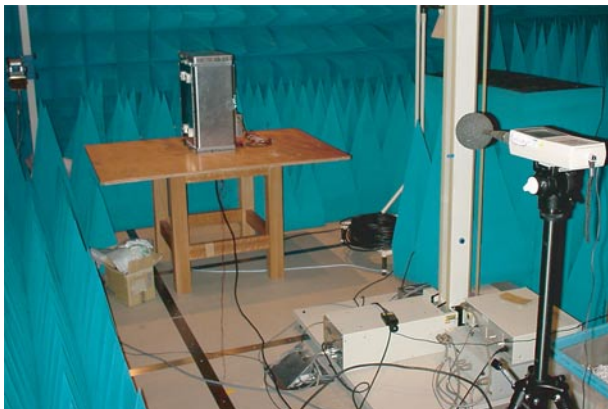
写真2 騒音測定状況 Experimental setup for noise measurement.
