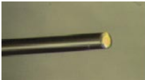
図10 ファイバ端のWDMフィルタ WDM filter evaporated on the facet of angled polished fiber.
