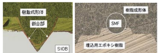
図9 樹脂成形体突起部とシリコン基板のV溝かん合部断面(左)及びΩ溝部断面(右) Cross-sections of the V-groove alignment on silicon substrate (left), and the Ω-shape groove of plastic mold (right).
