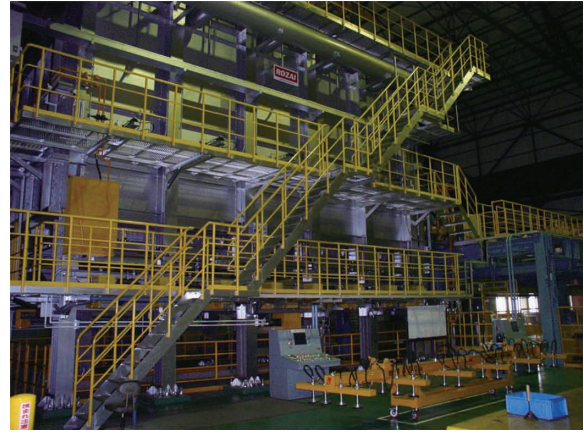
図2 2号焼入炉 No.2 quenching furnace.
