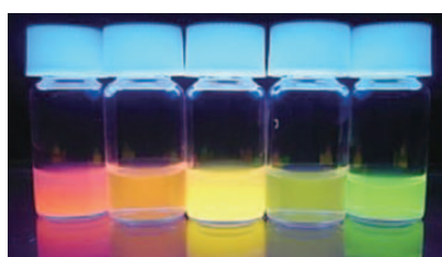
図2 Quartz Dotコロイド Colloidal dispersions of Quartz Dot.
