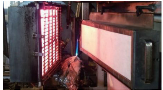
図3 火炎伝搬性試験機、加熱装置(左)と点火パネル(右) Flame propagation testing equipment, heating device (Left) and the ignition panel (Right).
