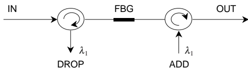
Figure 4 Schematic of OADM with fiber Bragg grating
