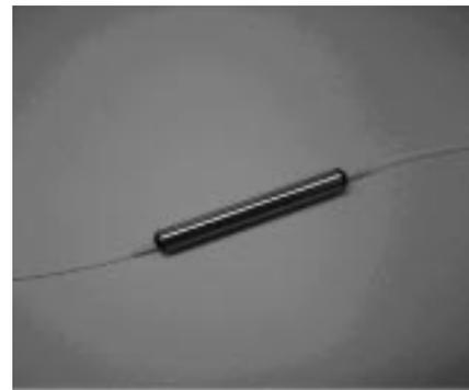
Figure 10 Appearance of etalon-type gain-flattening filter
