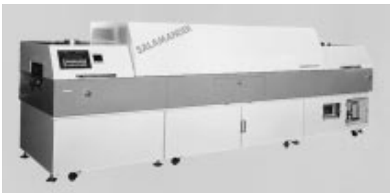
Figure 1 SALAMANDER-XN nitrogen-atmosphere reflow oven
