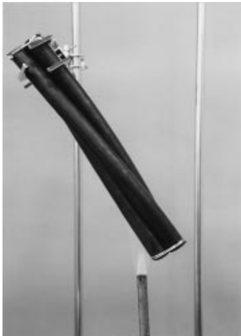
Photo 3 Flame retardance test (JIS C 3005)
