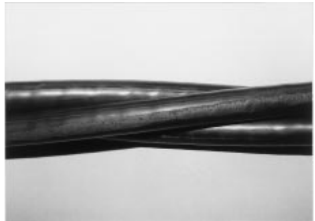
Photo 4 Appearance of a cable after damage resistance test
