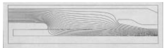
Figure 4 Result of electric field analysis for designing splice body
