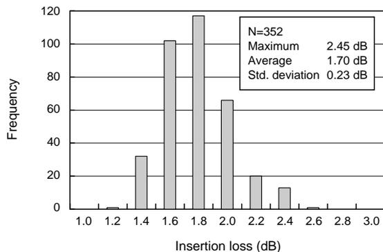
Figure 4 Optical coupler insertion loss, A port to B port (1550 nm)
