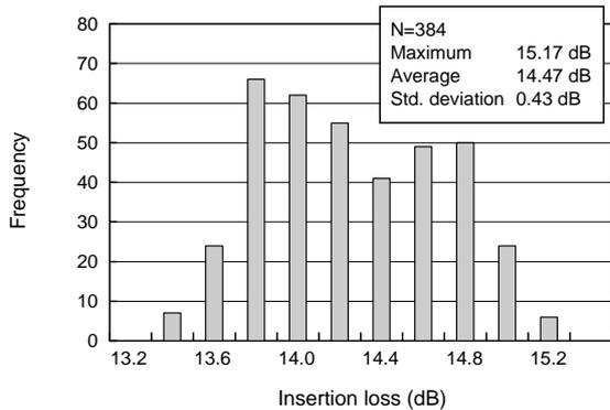
Figure 7 Optical jumper unit insertion loss, A port to B port (1310 nm)
