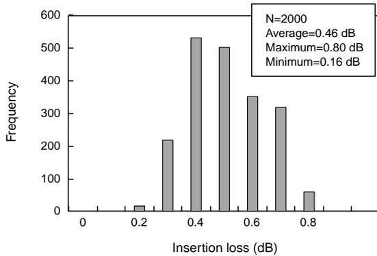
Figure 13 Fiber selector insertion loss
