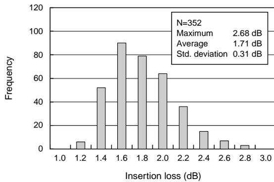
Figure 3 Optical coupler insertion loss, A port to B port (1310 nm)
