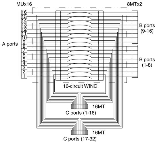
Figure 2 Configuration of optical coupler unit
