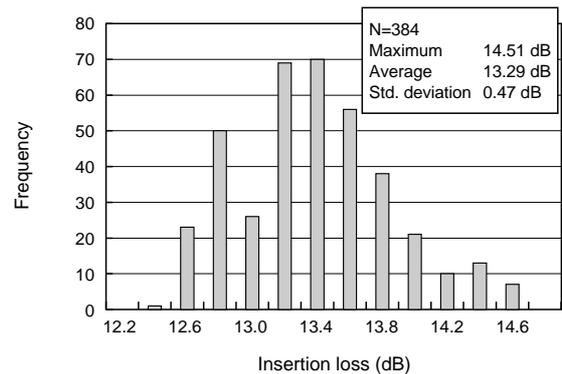
Figure 8 Optical jumper unit insertion loss, A port to B port (1550 nm)
