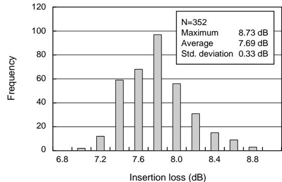
Figure 5 Optical coupler insertion loss, A port to B port (1650 nm)
