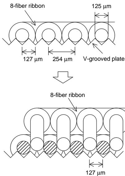
**Figure 10 Alignment of fixed-fiber array**
