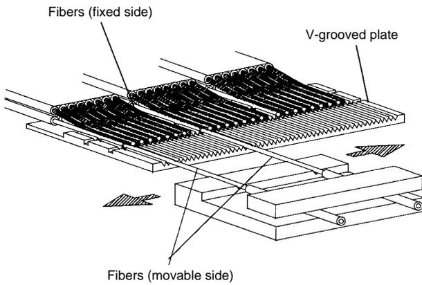
**Figure 9 Basic structure of optical switch**
