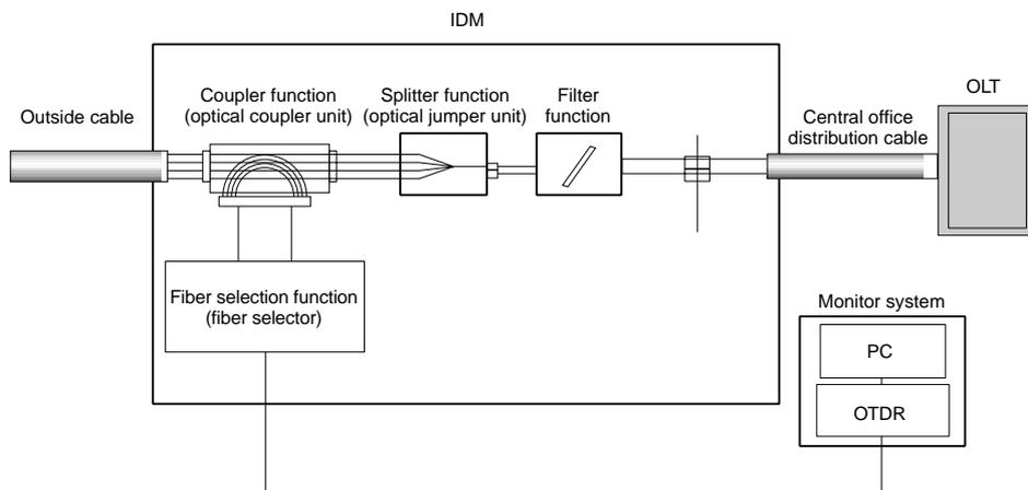
Figure 1 Configuration of optical fiber distribution management system
