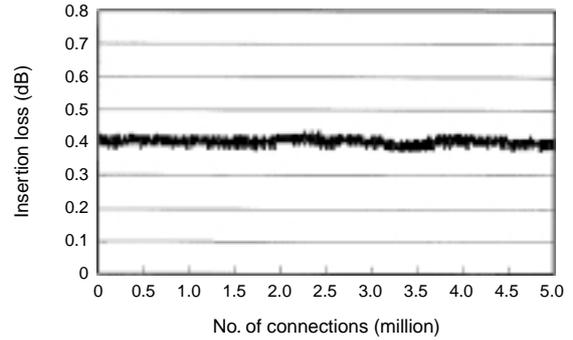
Figure 15 Fiber selector durability
