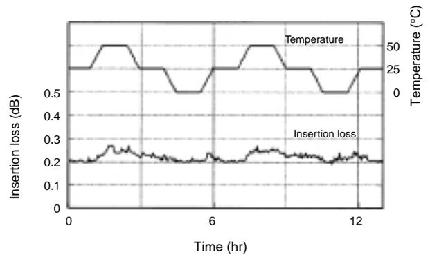
**Figure 11 Repeatability of insertion loss in heat-cycle tests**
