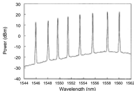
Figure 7 Output spectrum of EYDF
