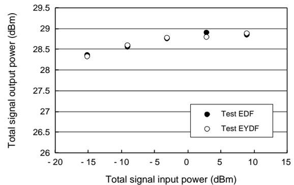
Figure 5 Signal input power dependence of output signal power
