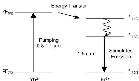
Figure 1 Model of energy levels in an Er-Yb system
