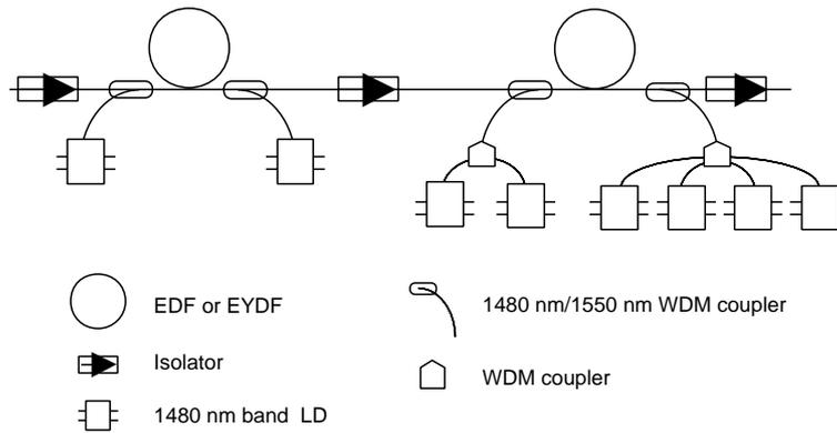
Figure 4 Schematic diagram of WDM amplifier
