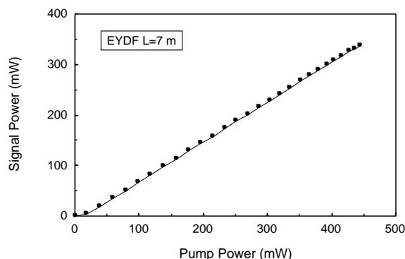
Figure 3 Pumping power dependence of output signal power for EYDF pumped at 1480 nm
