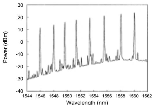
Figure 6 Output spectrum of EDF
