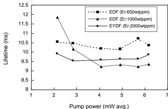
Figure 2 Pumping power dependence of fluorescence lifetime
