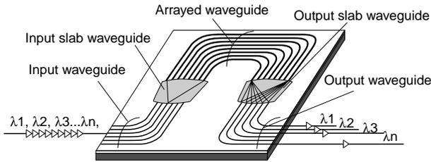
Figure 2 Waveguide circuit structure of AWG.
