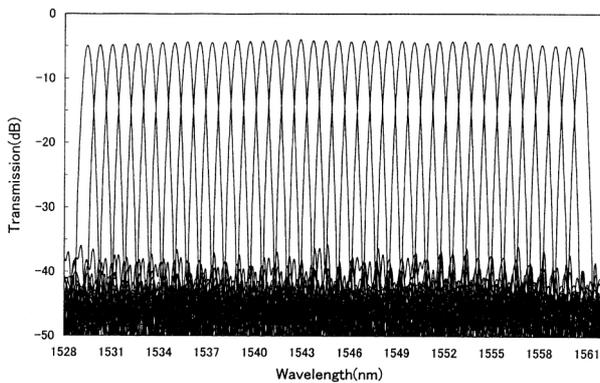
Figure 6 Typical transmission spectrum of 100-GHz, 40-ch heater-control AWG module.
