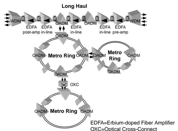
Figure 1 Schematic of a DWDM optical communication network.
