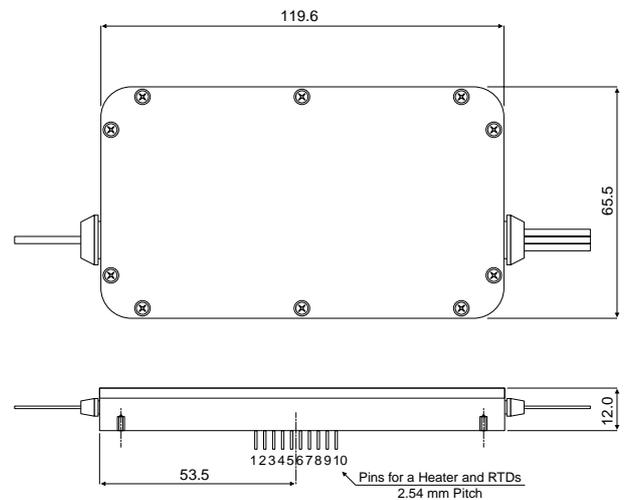
Figure 4 Dimensions of 100-GHz, 40-ch heater-control AWG module.
