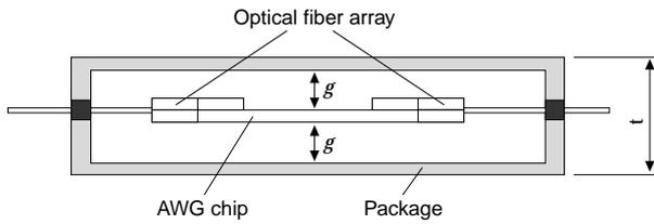
Figure 3 Cross-sectional view of AWG module.
