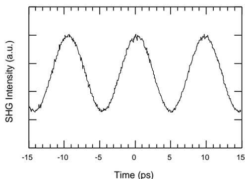
Figure 3 Autocorrelation trace of fiber input beat pulse.
