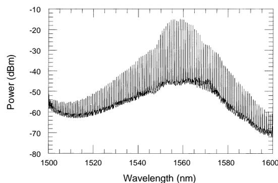
Figure 8 Optical spectrum of DI-NOLM output pulse.
