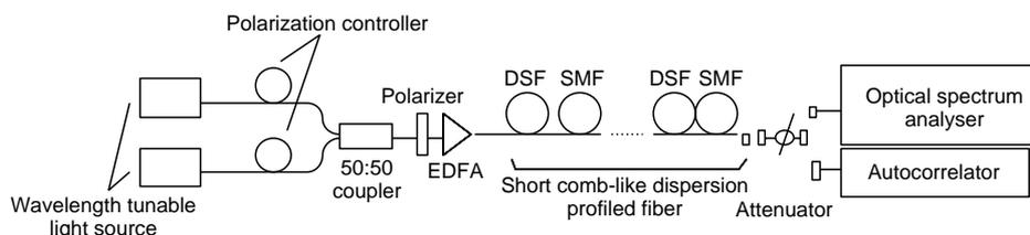
**Figure 2** Experimental setup.
