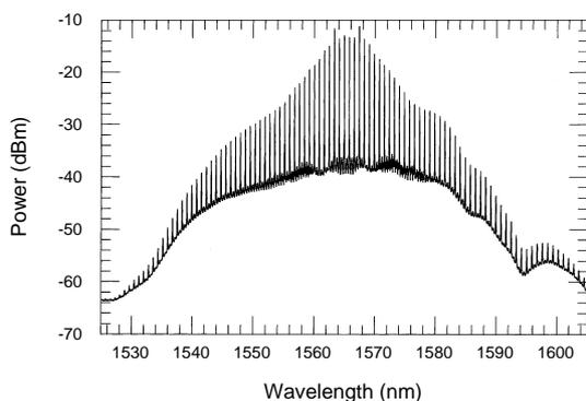
Figure 4 Optical spectrum of output pulse.
