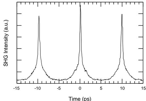
Figure 5 Autocorrelation trace of output pulse.
