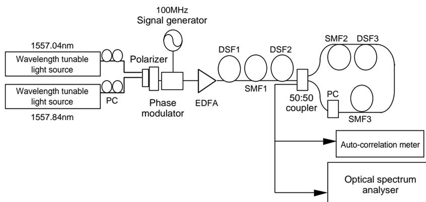
Figure 6 Experimental setup. P.C.: polarization controller
