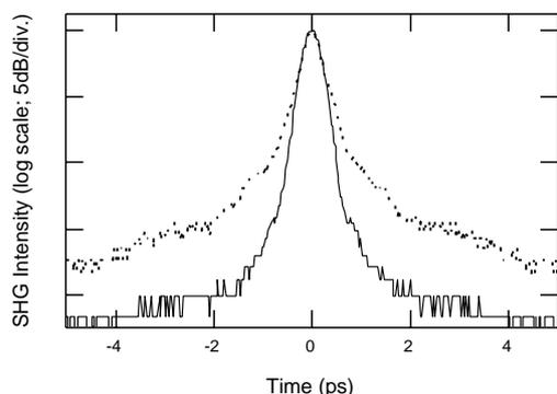
**Figure 9** Autocorrelation trace of DI-NOLM output pulse, showing loop mirror output (solid line) and SMF3 output clockwise propagation in the DI-NOLM (dashed line).
