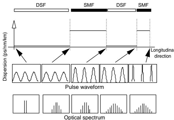
**Figure 1** Pulse compression process using comb-like dispersion profiled fiber. (Example of two pairs of DSF and SMF)
