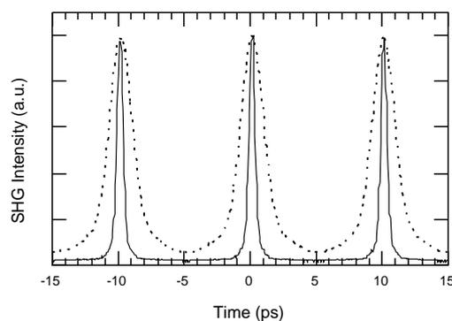
Figure 7 Autocorrelation traces of DI-NOLM input (dashed line) and output (solid line) pulses.
