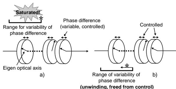
Figure 4 Control procedure for endless tracking (unwinding).
