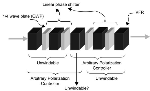
Figure 5 5-stage polarization controller with VFRs.
