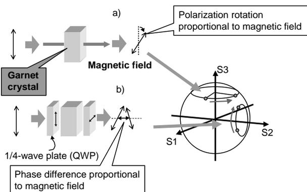
Figure 1 Operating characteristics of VFR.
