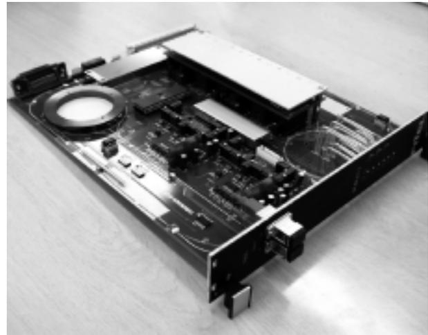
Figure 12 PMD compensator.
