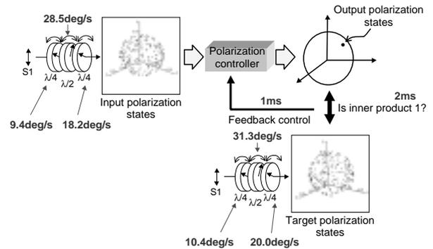
Figure 9 Configuration schema of simulation.
