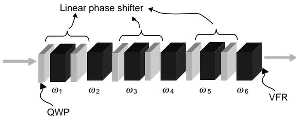
Figure 7 6-stage polarization controller with VFR.
