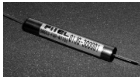
Figure 5 Appearance of TFF-based optical combiner module.
