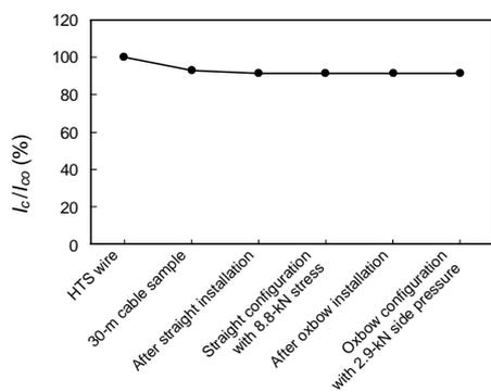
Figure 6 Critical currents of a cut-off sample after cable manufacture and installation.
