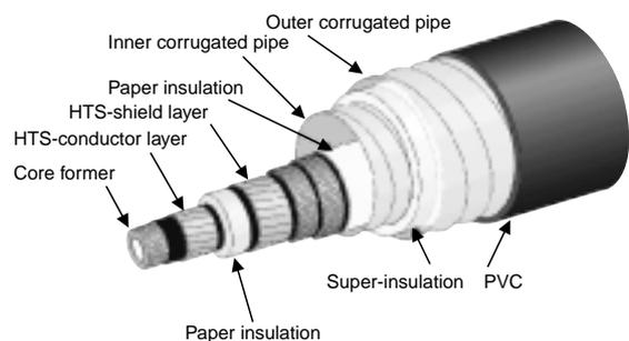
**Figure 1** HTS power cable with single core and cryogenic dielectric.
