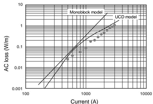
Figure 4 Results of measurement of AC losses in HTS conductor.
