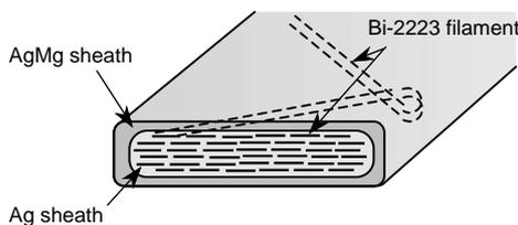
Figure 3 Structure of twisted filament tape.
