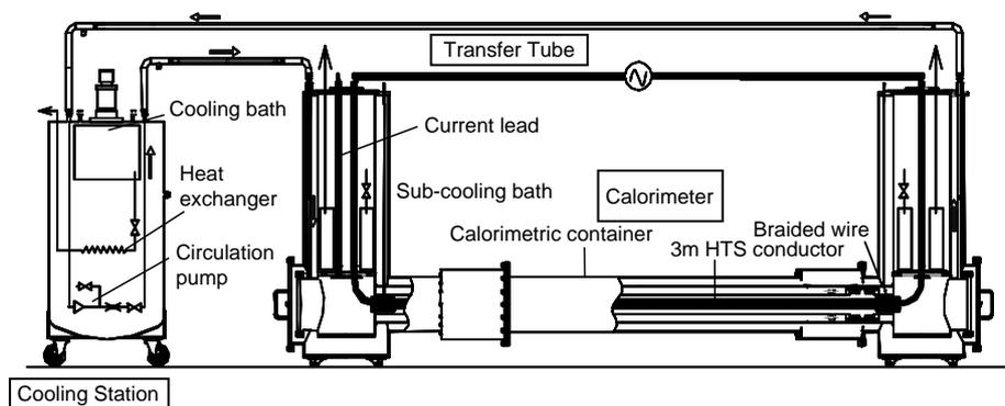
Figure 5 Calorimetric device for measuring AC losses in HTS conductor.
