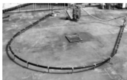
Photo 2 30-m HTS cable installed in oxbow shape in Furukawa Electric's laboratory for tests.
