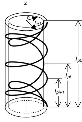
Figure 2 Closed circuit enclosed with an i layer tape and an i+1 layer.
