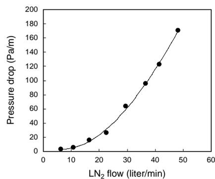
Figure 7 Pressure drop of single-phase LN<sub>2</sub> flowing into 30-m long HTS cable.
