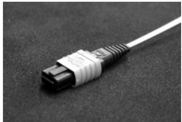
Photo 1 Super low-loss MPO8 optical connector.
