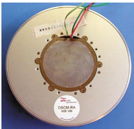
Figure 7 Raman amplifier module with integrated DCF.
