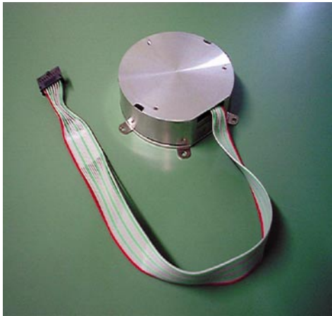
Figure 5 Outside view of Raman pumping laser module.
