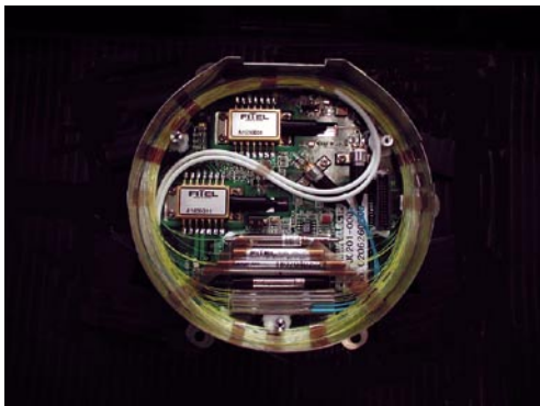
Figure 6 Inside view of Raman pumping laser module.
