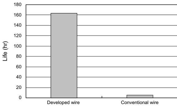
**Figure 2 Comparison of life under inverter surge between the developed and conventional wires.**
