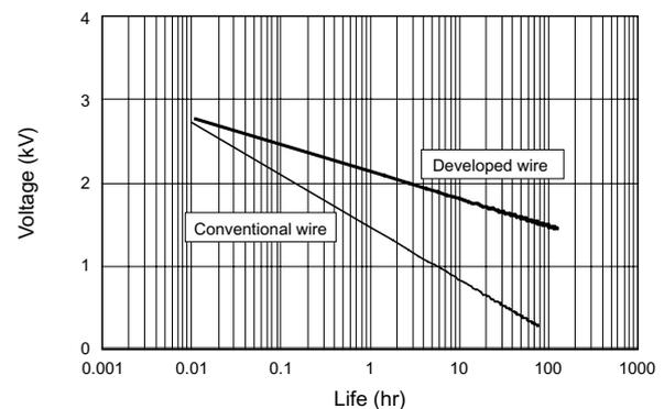
**Figure 1 Comparison of V-t characteristics between the developed and conventional wires.**
