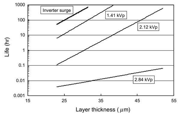
**Figure 4 Layer thickness dependence of the sinusoidal wave life under selected voltages and the life under inverter surge.**
