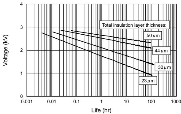
**Figure 3 Comparison of V-t characteristics of the developed wire with different insulation layer thicknesses.**
