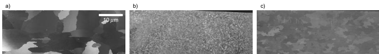
Figure 11 Macrostructures of fin stocks after heating for brazing. a) Fin stock developed here, b) Al-Fe-Ni-Si fin stock by DC method, c) 3000-series alloy
