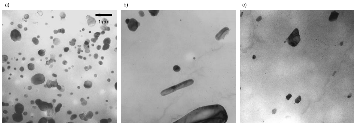
Figure 10 TEM images of fin stocks after heating for brazing. a) Fin stock developed here, b) Al-Fe-Ni-Si fin stock by DC method, c) 3000-series alloy
