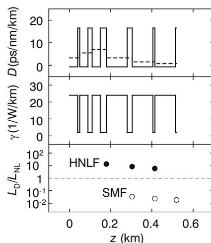
Figure 3 Profiles of dispersion ( $D$ ) and nonlinearity  $\gamma$ , and the ratio of dispersion length ( $L_D$ ) to nonlinear length ( $L_{NL}$ ). Broken line shows the averaged dispersion for each pair ( $D_{\text{ave}}$ ).
