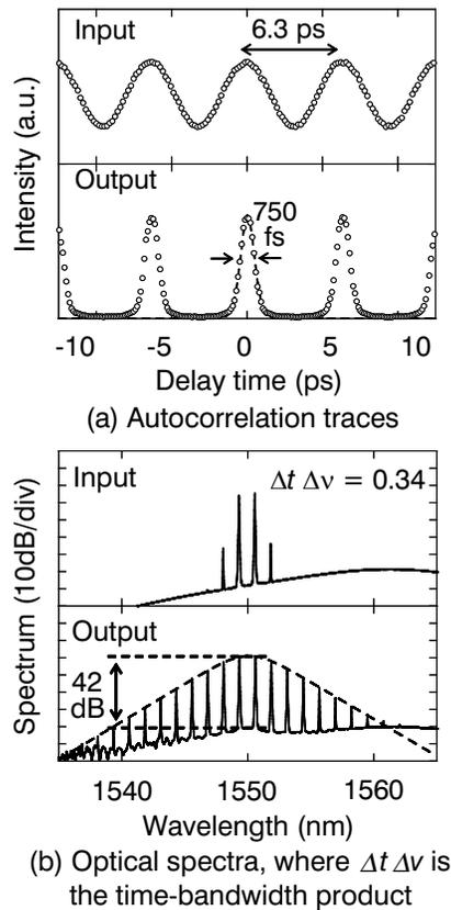
Figure 4 Input and output pulse trains of CDPF.
