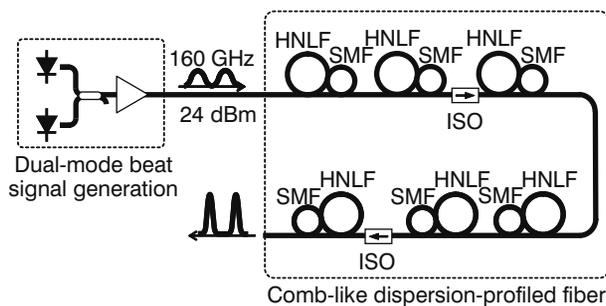
Figure 2 Experimental setup for 160-GHz soliton train generation using CDPF.
