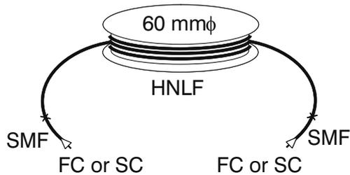
**Figure 5** Splicing of SMF to the ends of the HNLF, and the input and output connectors.
