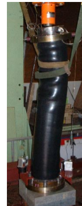
Photo 3 Axial compression test where buckling occurred.
