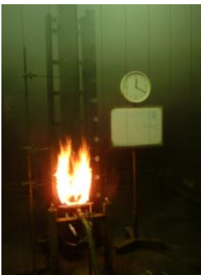
Photo 8 Inflammability test, burning sample.
