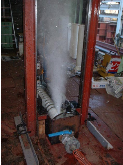
Photo 6 S4 test of all-PE pipe.
