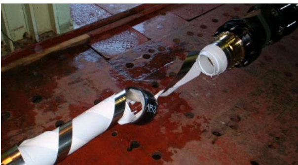
Photo 5 Tensile test where breakdown occurred.
