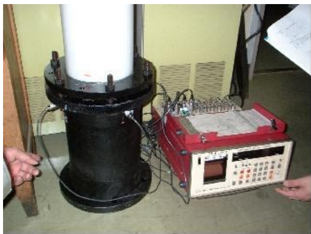
Photo 6 Test for the relaxation of sealing surface pressure.
