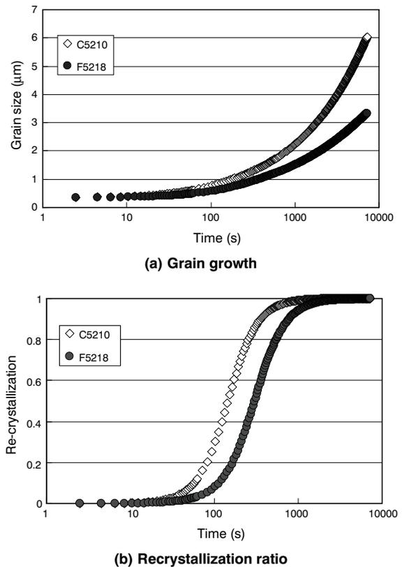
Figure 6 Calculated grain growth and recrystallization ratio.
