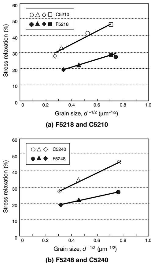
Figure 3 Stress relaxation characteristics of selected alloys.
