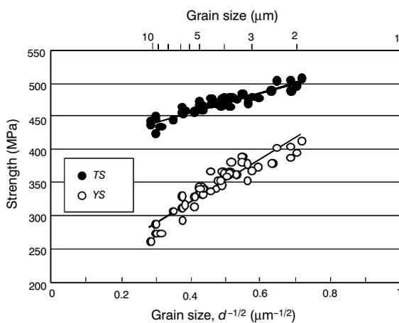
Figure 1 Grain size dependence of strength of F5218.
