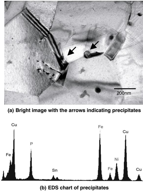
Figure 5 TEM image and EDS analysis of F5218.
