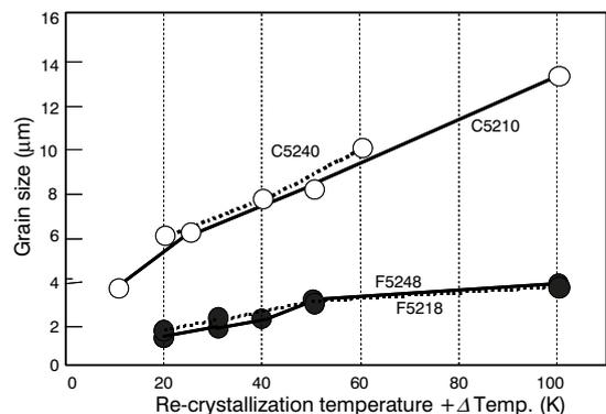
Figure 4 Relationship between grain size and heat treatment temperature.
