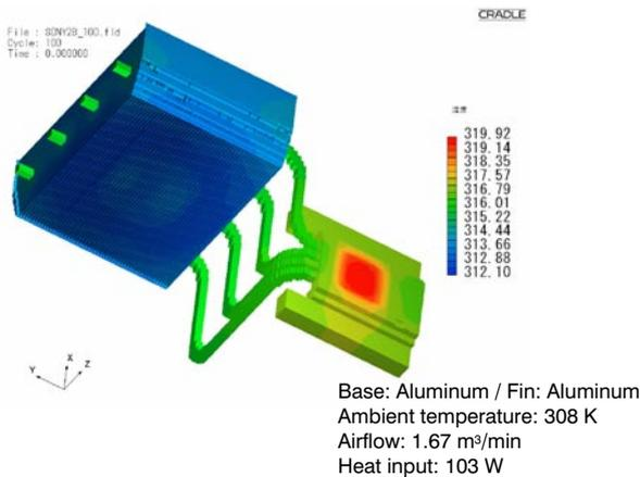
**Figure 11 Temperature distribution of heatsink. (by calculation)**
