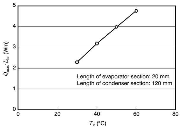
Figure 9  $Q_{max} \cdot L_{hr}$  of L-shaped heatpipe.
