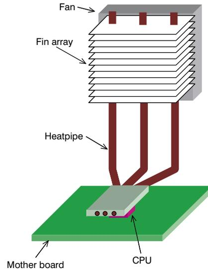
Figure 4 Schematic diagram of HP-RHS.
