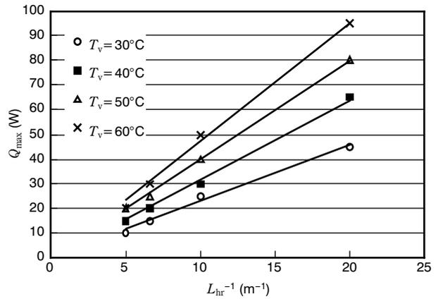
Figure 8  $Q_{max}$  of L-shaped heatpipe under various conditions.
