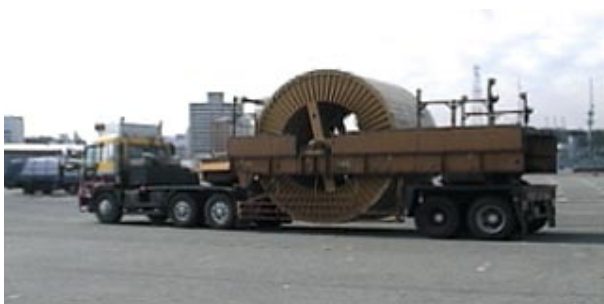
Figure 4 Transportation of the 500-m HTS cable.
