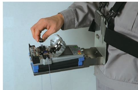
Photo 3 High portability with a foldable hinged working table.
