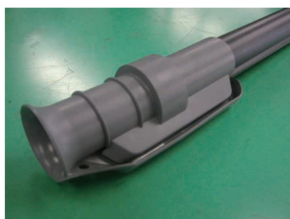
Figure 24 Overhead line protector.
