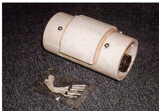
Figure 38 “Fusion Joint”, where conductors are welded without forming an electrical connection.
