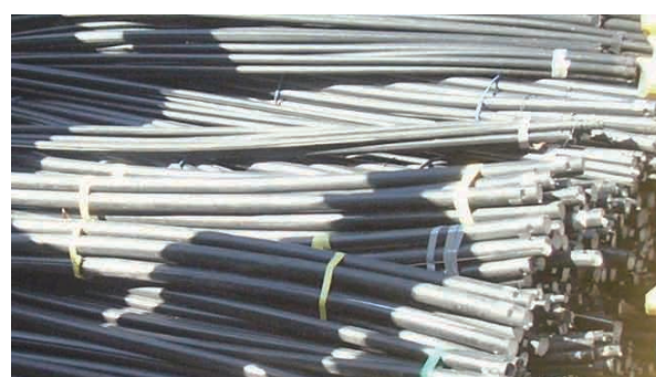
Figure 27 Removed overhead line protector.
