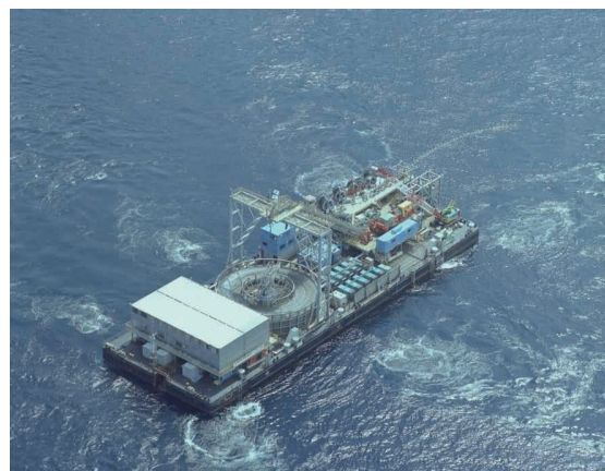
Figure 8 Cable laying ship "Tenzan" with DPS function, built by using pure domestic technologies.
