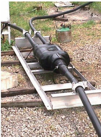
Figure 12 154-kV compact Y-branch joint, measuring 300 mm x 600 mm x 1,500 mm.
