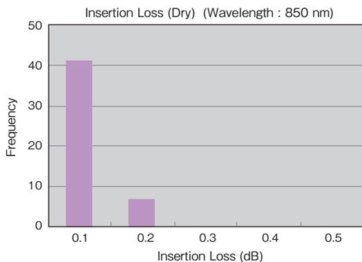
Figure 11 Connection loss of the  $\mu$ -Joint-MU multi-mode type plug in adaptor.
