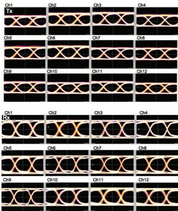
Figure 17 Optical and electrical waveform of 5 Gbps, 12channels transmitter and receiver module.
