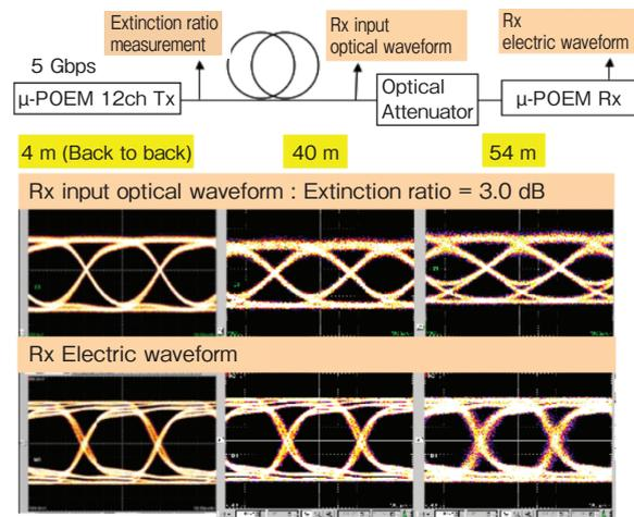
Figure18 Optical waveforms of 5 Gbps x 12 channel transmitter module over ThreadWave MM.
