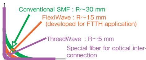
Figure 4 Comparison of fiber bending radius.
