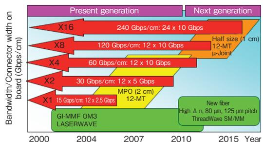
Figure 2 Expectation of bandwidth per optical connector width of one centimeter.
