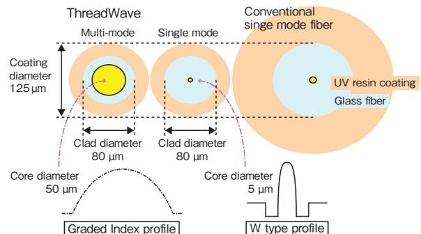
Figure 5 Cross-section of the ThreadWave fibers.
