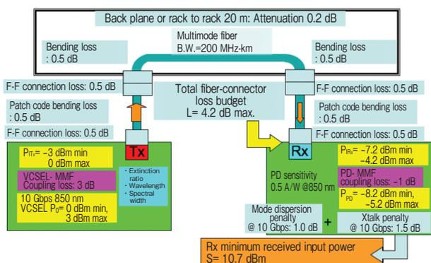
Figure 1 Structure and transmission loss budget design of Optical-Interconnection System.
