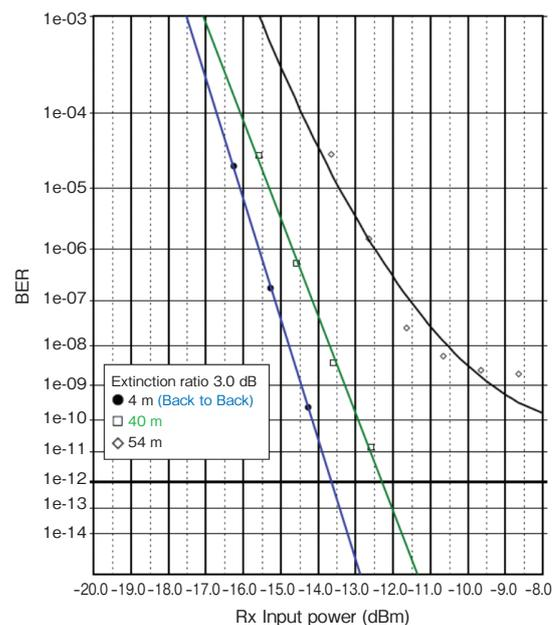
Figure 19 Bit error ratio test of the 5 Gbps  $\mu$ -POEM V-pack type over ThreadWave MM fiber.
