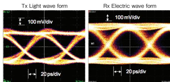
Figure 20 10-Gbps Waveform of  $\mu$ -POEM R-pack type (Left: Tx optical, Right: Rx electrical).
