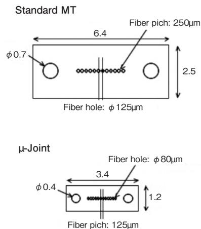
Figure 8 Cross-section of conventional MT ferrule and μ-Joint ferrule.
