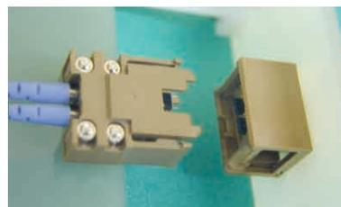
Figure 12  $\mu$ -Joint-MU backplane connector (Left: print board connector, Right: backplane connector).
