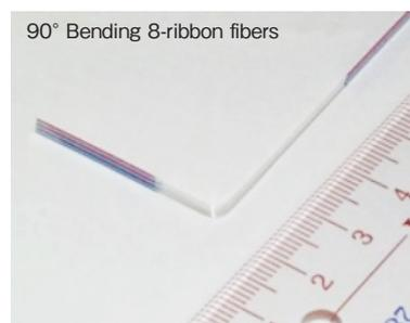
Figure 13 90-degree bending fiber ribbon.
