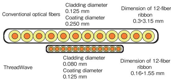
Figure 6 Comparison of cross-sections: Conventional 12-fiber ribbon and ThreadWave 12-fiber ribbon.
